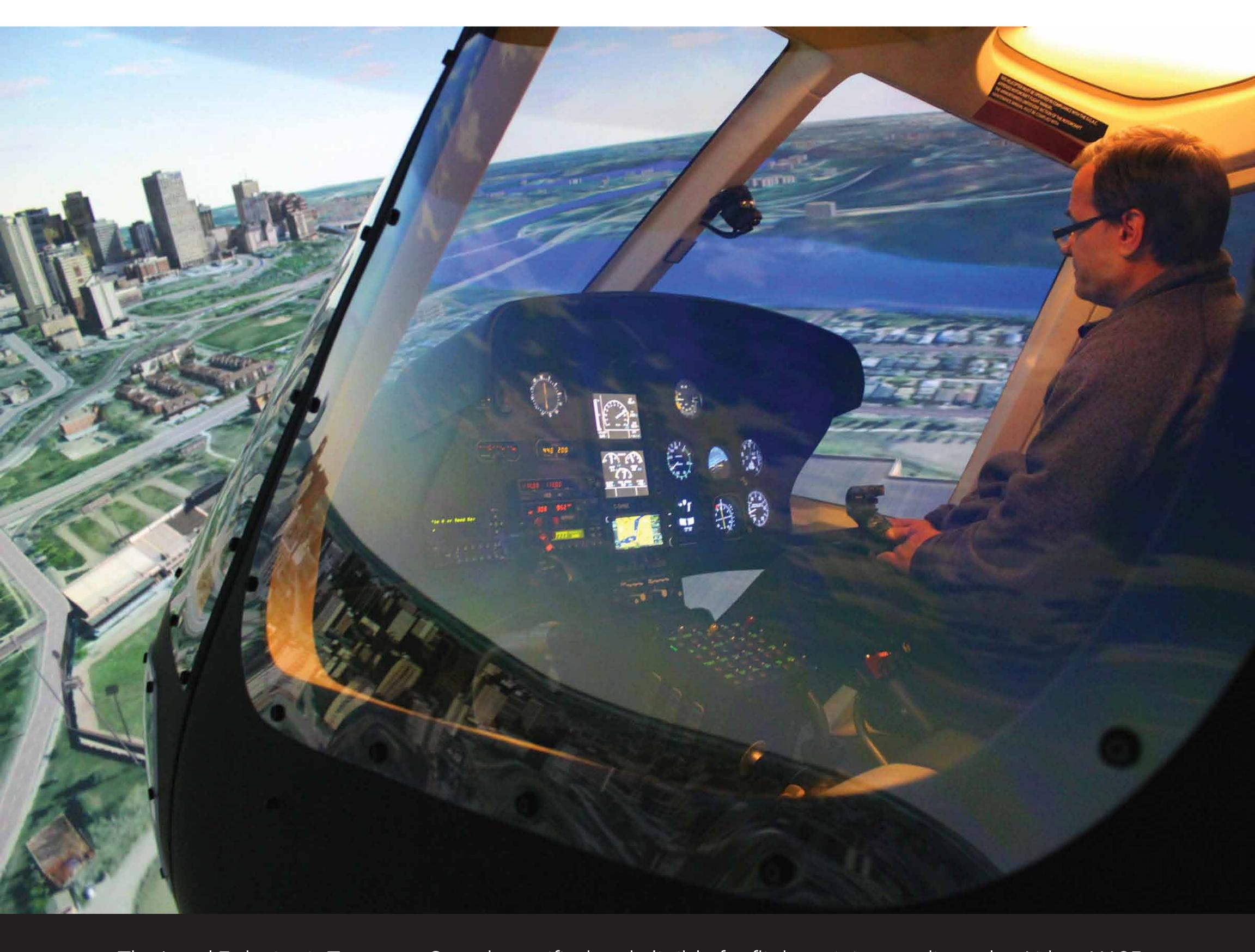
The Level 7 device is Transport Canada certified and eligible for flight training credit on the Airbus H125 and AS350B2 helicopter variants. The device is at the leading edge of synthetic training technology and offers extensive user defined LOFT scenarios and AS350 emergency procedure training.
